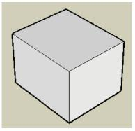
2. A box is boring, so we'll make it more interesting. Use **Scale** on the top face to shrink it. (Press Ctrl / Option while using **Scale** to scale about the center of the face.)
