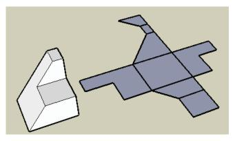
This one is especially tough - a box with a smaller box cut out at one corner.
