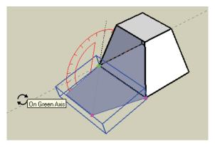
7. Keep unfolding faces one by one. When you get to this stage, you have two connected faces that need to be unfolded together. (If you just unfold the larger vertical face, the top face will be left hovering alone in space.)
