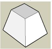
3. You can't unfold the faces like this, because they are all stuck together. To separate them, each face must be a group. Select a face plus its edges (while using **Select**, you can double-click a face for this). Right-click on the face, and choose **Make Group**.
